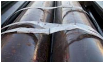
3. Correctly Applied and Crimped Seal
